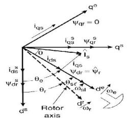
Figure 3: Phasor Representation of Indirect Vector Control IM.
